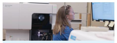
AgSource Laboratories uses three generations of Agilent ICP-OES instruments to analyze soils, plants, and manures to support farming activities in Wisconsin, USA.
