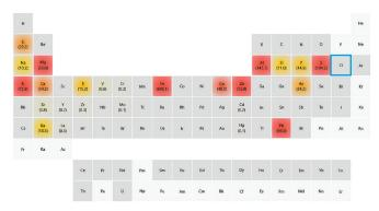
Elements shaded red are in high concentration, orange are in mid-range concentration, and those in yellow are in low concentration. Unshaded elements are not at detectable levels in the sample. In this case, Cl is missing, indicating that HCl was not used during sample preparation.
