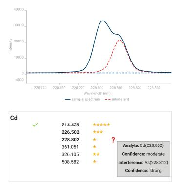
IntelliQuant Star ranking output for Cd. A five-star ranking with green check mark indicates Cd 214 wavelength to be the best. The red question mark indicates there is an issue on Cd 228, and the pop-up tip indicates the Cd 228 result has only moderate confidence as it has a strong arsenic interference.
